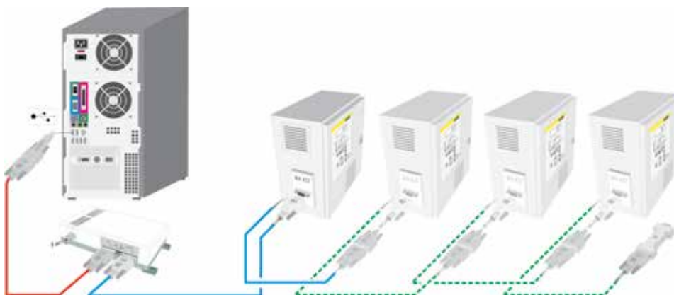
Extendable for connection of up to 16 furnaces
