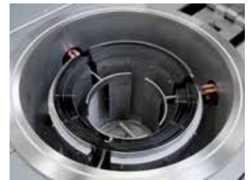
Cylindrical retort with tungsten heating
