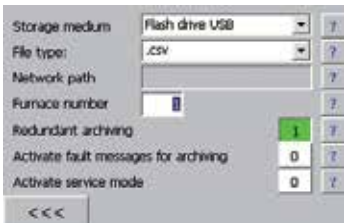
NTLog Basic for data recording of Nabertherm Controllers
