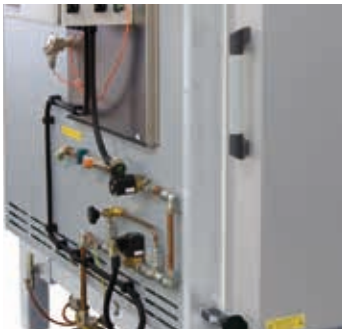
Gas lines and thermocouple at the furnace
