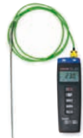
Temperature gauge for RAKU 100, easy to operate, NiCr-Ni temperature sensor, display range 20 - 1200 °C, optional connection of second sensor with display changeover
