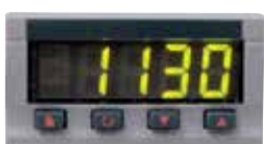
Over-temperature limit controller
