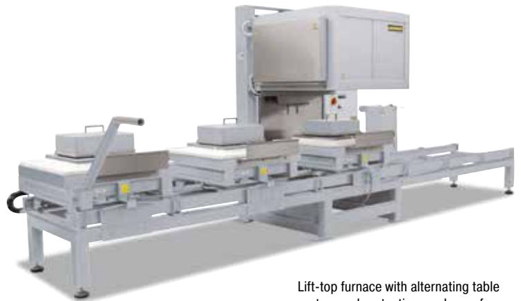
Lift-top system H 245/LTS with cooling station and table changing system
