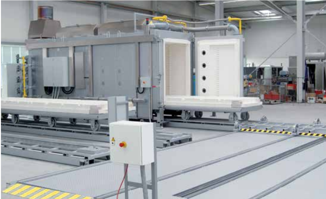
Combi furnace system consisting of one gas-fired furnace WB 11000HS and two additional bogies incl. bogie transfer system and incl. necessary park rails
