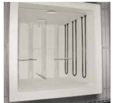
Fresh air injection through perforated injection tubes with debinding package II
