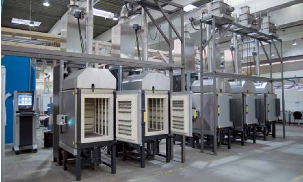
Production system consisting of five combi chamber furnaces N 300/HDB with debinding package II with catalytic afterburning
