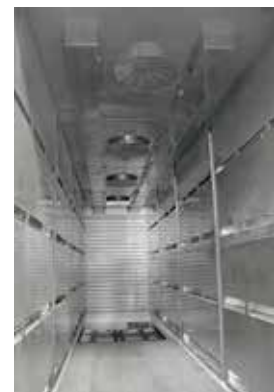
Furnace chamber with air baffle plates
