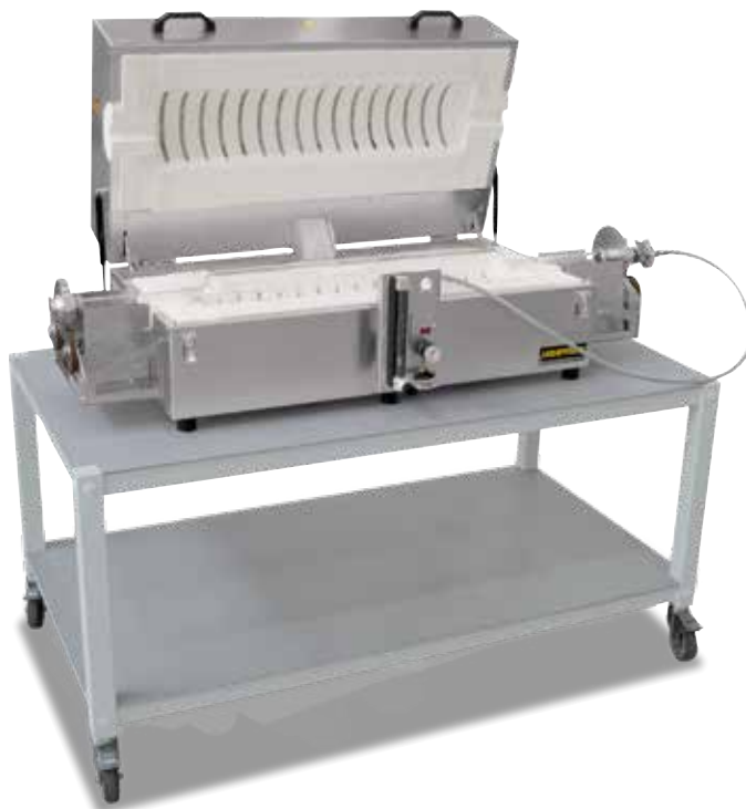
RSR-B 120/750/11 as tabletop version for batch operation
