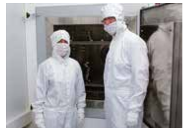
Air circulation furnace N 250/65 HAC for clean room Class 100 with charging door to the clean room
