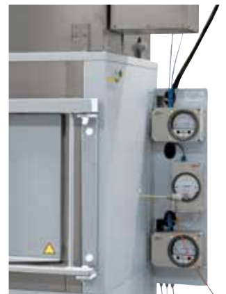
Display of pressure and volume flow with debinding package II
