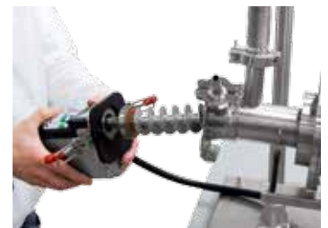
Screw-conveyor with adjustable speed
