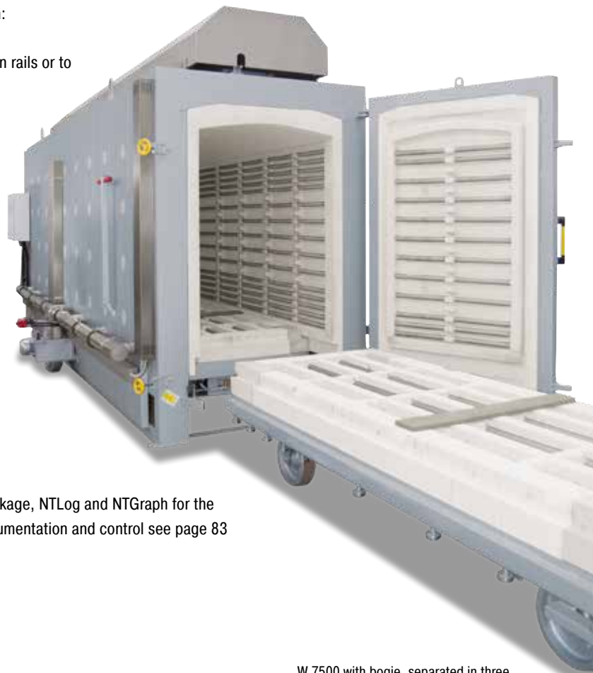
W 7500 with bogie, separated in three parts
