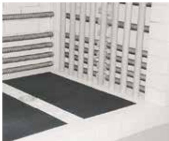
Injection of preheated air through perforated ceramic tubes
