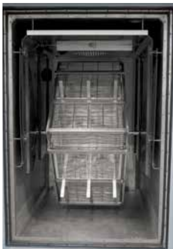
Motor-driven rotary rack with baskets for moving the charge during heat treatment
