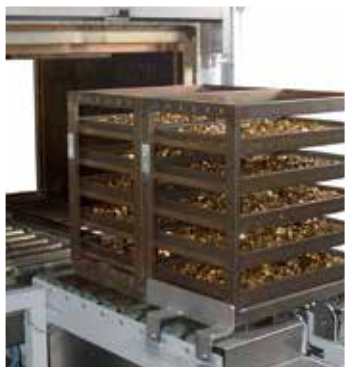
Continuous belt furnace for bulk materials in baskets
