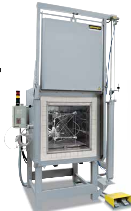
Holding frame for measurement of temperature uniformity
