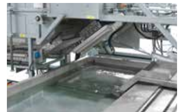
Drop bottom for quenching within 5 seconds
