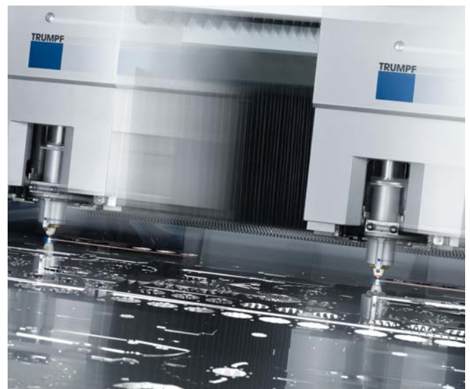
Twice the productivity with two cutting heads.
