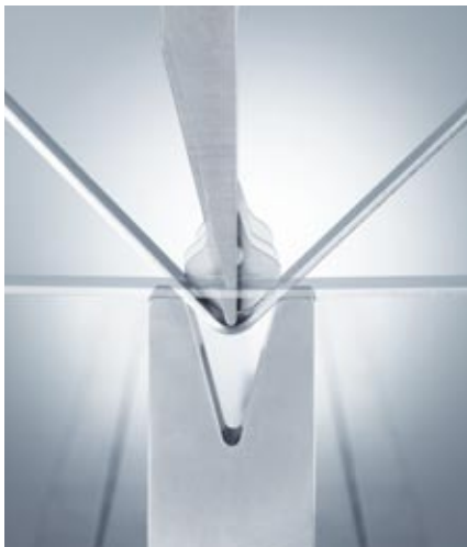
Automatic bending with angle sensor ACB.
