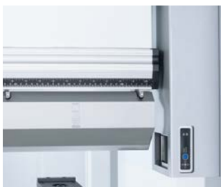
The BendGuard can easily be pushed to the rear making it possible to load from the side.
