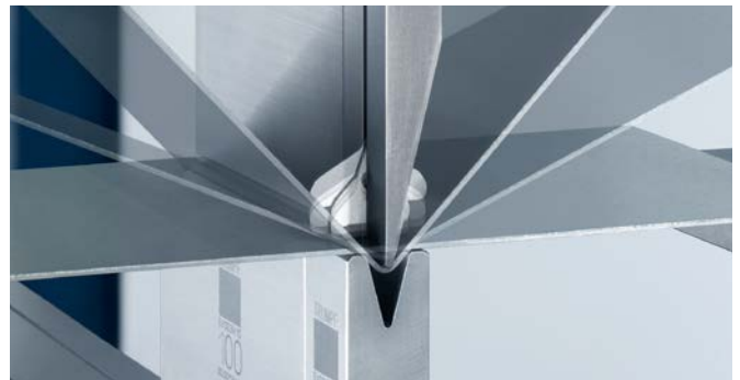
Tactile angle measuring system ACB Wireless.
