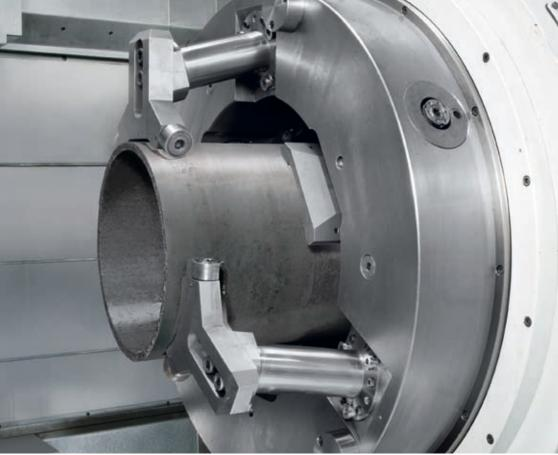
Pipe ends are threaded by rotating the pipe in our Danobat TT model lathes. These machines are designed with a modular concept utilizing Finite Element Analysis. The main features are as follows:
