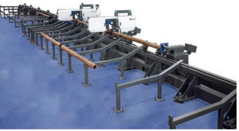
The pipe machining process begins with the cutting of the ends, where we incorporate fully automated lines with two Danobat CP sawing machines that can move along a slide in order to adjust pipe length according to your specifications.
